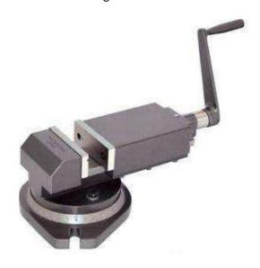
86.2 Total Height: 343 mm ±2 mm 86.3 Base Length: 165 mm ±2 mm 86.4 Base Width: 165 mm ±2 mm 86.5 Height: 120 mm ±2 mm 86.6 Jaw Width: 100 mm ±2 mm 86.7 Jaw Opening: 1002 mm ±2 mm 86.8 Jaw Depth: 38 mm ±2 mm 86.9 Jaw Hardness: 55 HRC
