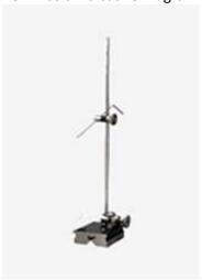
16.2 Base should be made from case hardened steel, ground on bottom and at one end.
