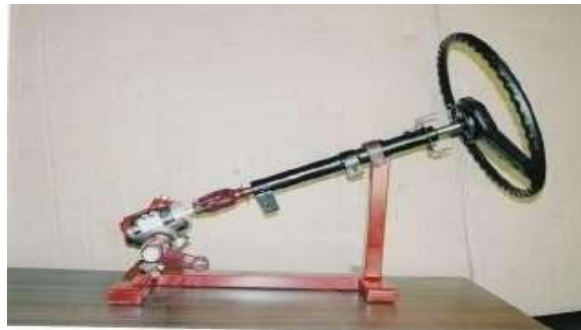
2. Worm & Roller steering assembly with drop arm
