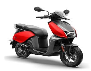
72.2 Range: 110Km/Hr., Motor Power: 6 Kw, Motor Type: PMSM,
