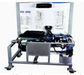
84.2 The device should be designed based on latest technology with Multi Point Fuel Injection System. The trainer should be able to simulate engine start up, speedup, slowdown and other actions so as to illustrate the structure and working principle of MPFI engines.
