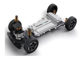
89.2 EV Four-Wheeler with High Voltage System with Lithium -Ion battery and Charger
