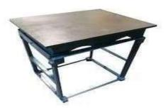
83.2 Total Length: 300 mm ± 1 mm 83.3 Total Width: 300 mm ± 1 mm 83.4 Total Height:  $350 \text{ mm} \pm 0.5 \text{ mm}$ 83.4 Plate Thickness: 25 mm ± 0.2 mm 83.5 Surface Plate Material: Cast Iron 83.6 Surface Finish: Precision Lapped Finish. 83.7 Uniformity in Hardness, Low Porosity, Non Magnetic, Easy To Clean. Rust Proof. Non-corrosive 83.8 Should be useful for measuring area flatness. 83.9 Suitable plywood cover should provided
