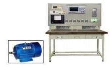
147.2 MOTOR: Synchronous motor 3 Phase, 3 HP, 415V, 50Hz, 4 Pole,
