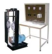
140.2 Basic Item Specification An integrated panel workbench consisting of instrument panel and working table should suitable for students to learn and perform various experiments of electrical related subjects. Instruments should internally electrically connected and should be fitted in the panel such that only front panel and necessary interfaces are easily accessible to use. Structure of workbench should be made up
